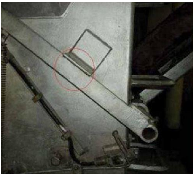
With door open, red circle indicates where crushing ensued
