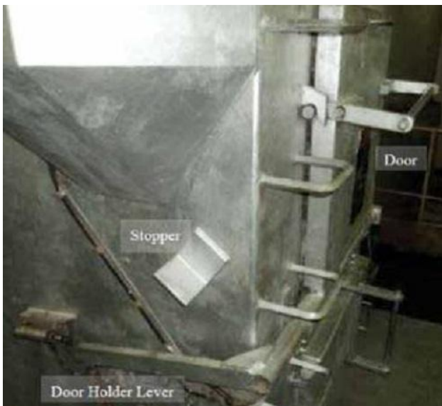
Incinerator with door closed
