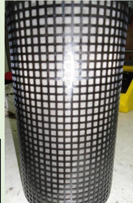
Filtro doble del motor principal – Main Engine Duplex filter
