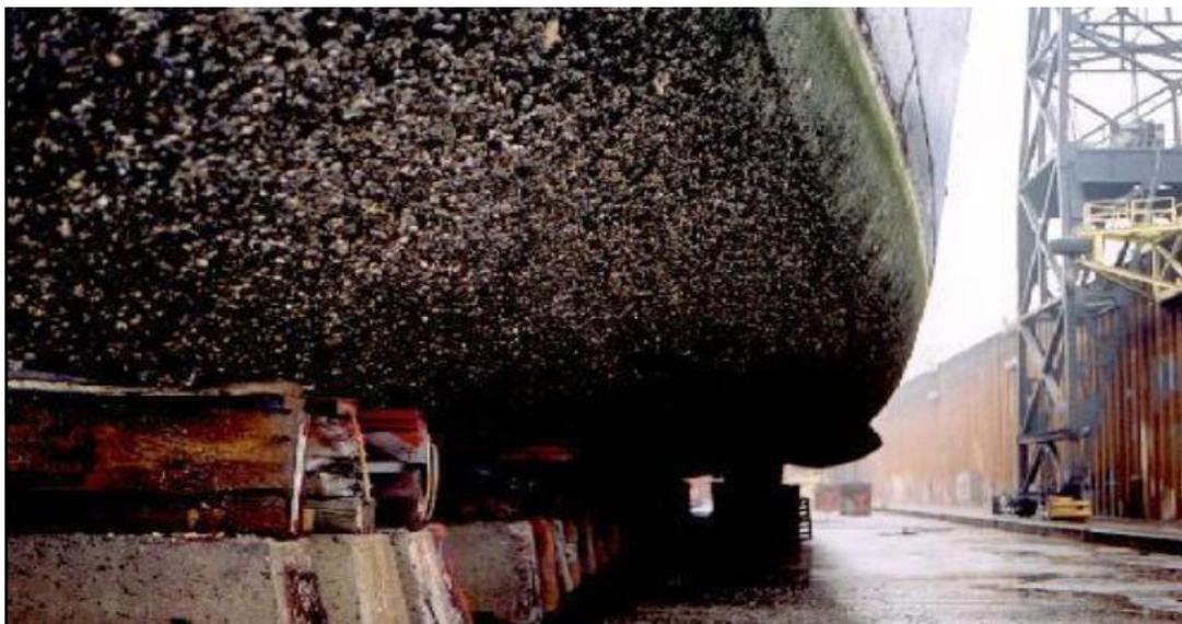
*Figura 8: HULL FOULING Causes and Consequences*
