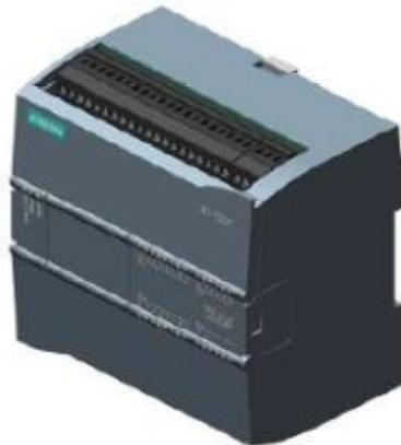
SIPLUS S7-1200 CPU 1214C AC/DC/RLY PARA ATMOSFERAS AGRESIVAS CON CONFORMAL COATING BASADO EN 6ES7214-1BG31-0XB0. CPU COMPACTA, AC/DC/RELE, ONBOARD I/O: 14 ED 24VDC; 10 SD RELE 2A; 2 EA 0 - 10V DC, ALIMENTACION: AC 85 - 264 V AC @ 47 -63 HZ, MEMORIA DE PROGRAMA/DATOS 75 KB
